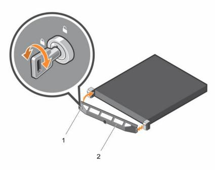
Figure 13. Removing and installing the front bezel
